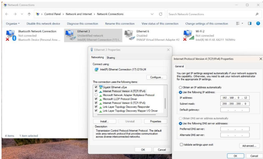
Fig 5.3 Set up IP of PC
