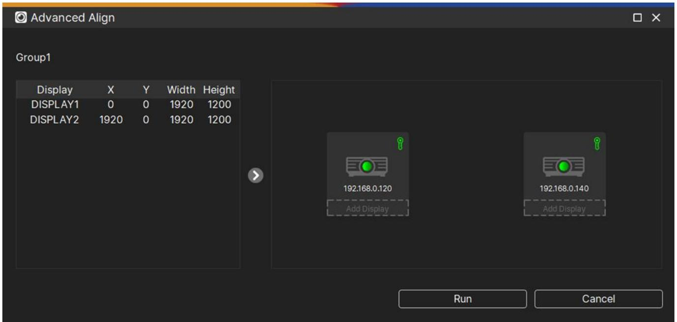
Fig 4.4.3 Drag display to the IP Layout
