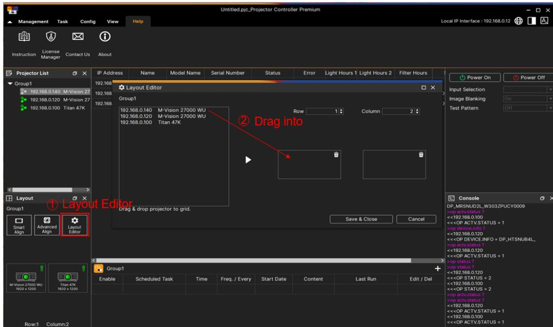
Fig 5.9 Set up IP Layout
