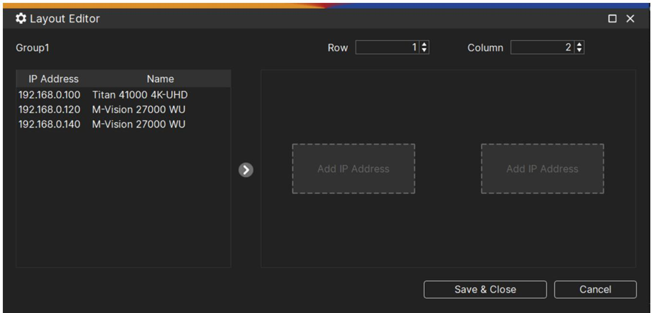
Fig 4.3.2 Drag IP to add IP Address in the right space
