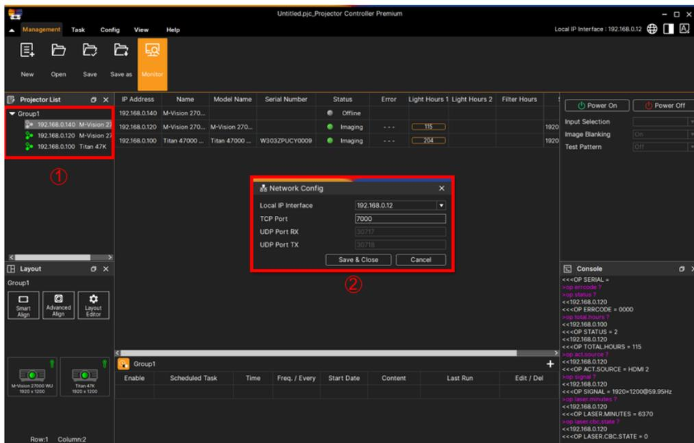
Fig 5.4 Set up projectors IP and Port
